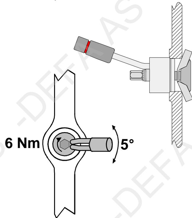
GB Drain off the coolant. Remove the indicated frost plug according to the table.
